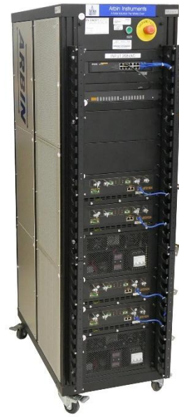
Fig. 1 Experimental Setup Using the Arbin LBT21024 System for Charge-Discharge Cycling of AGM and LiFePO 4 Batteries.
