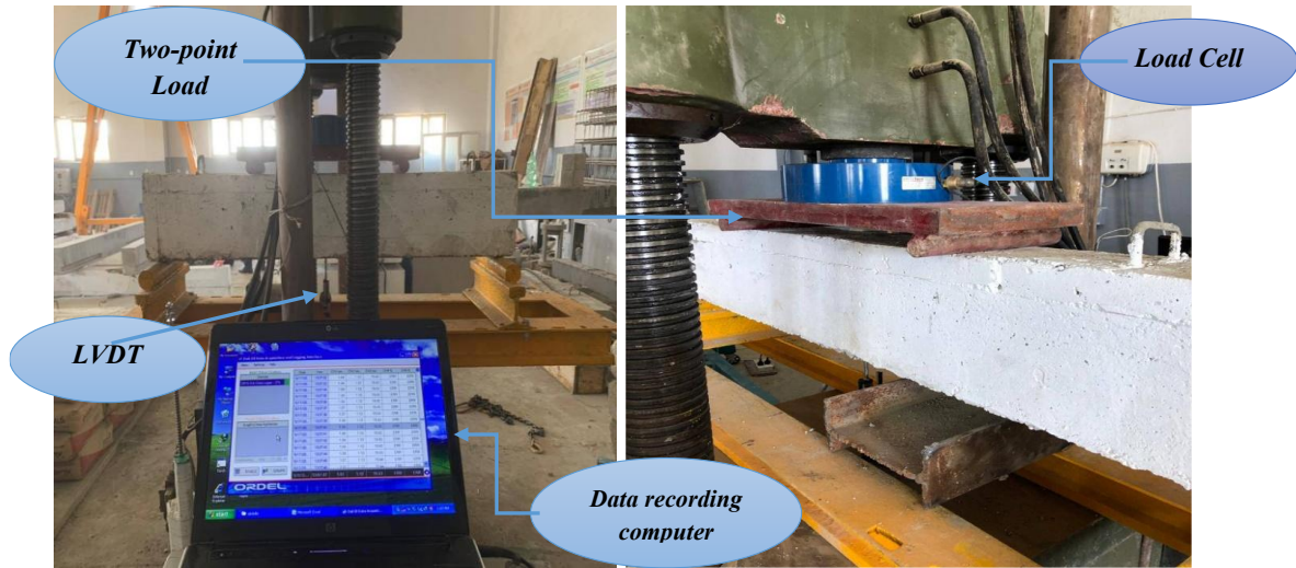
Fig.12 Details of the Testing of Beams.
