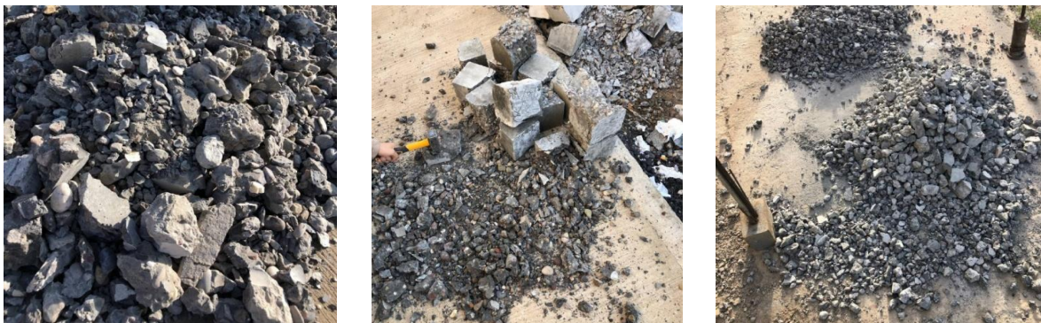
Fig. 3 Breaking Concrete Blocks into Small Pieces with a Gradient Similar to Natural Gravel.
