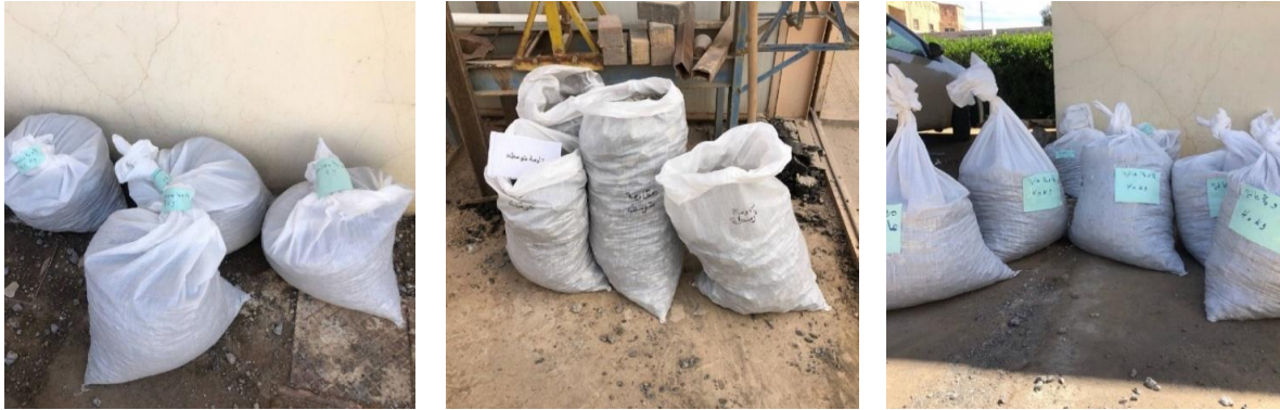
Fig. 5 Packing Recycled Concrete Aggregate into Bags.
