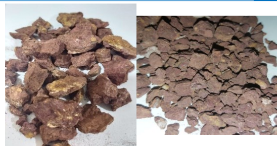
Fig. 3 Particle Size of the Sample (Hematite Ore), (a) Particle Size before Crushing (10mm), (b) Particle Size after Crushing (2mm).
