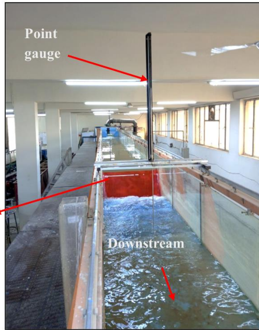
Fig. 1 Ogee Spillway Installed in the Laboratory Flume.
