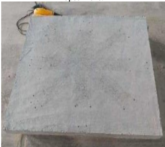
Fig. 10 Casting Concrete and Curing of Specimens.
